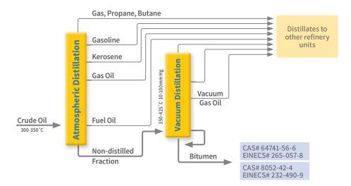
Figure 2. Schematic diagram of the distillation process
