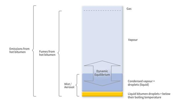
Figure 6. Schematic diagram of bitumen emissions
