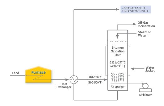
Figure 5. Schematic diagram of the bitumen oxidation process
