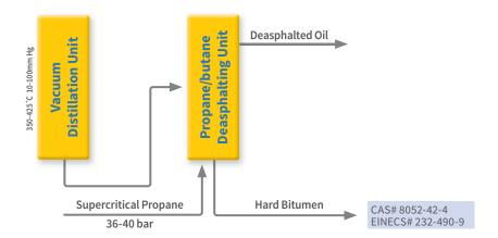
Figure 3. Schematic diagram of the propane deasphalting process
