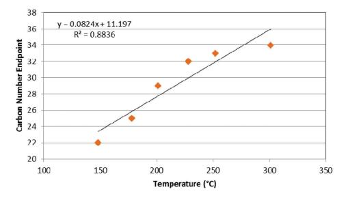
Figure 9. Fume Generation Temperature versus Carbon Number Endpoint
