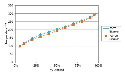
Figure 7. Boiling point distribution curves for bitumen emission samples - 50/70 (blue) 70/100 (orange).
